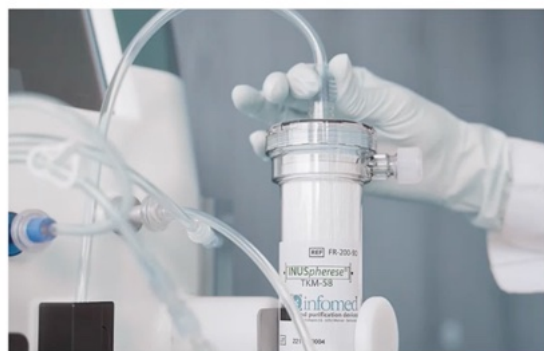
INUSpheres only allows particles smaller than 20-50 nm to pass through
